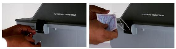
After installation of paper roll in the paper roll compartment of VVPAT, seal the latches of Paper Roll Compartment by passing a thread through holes provided on the latches using Address Tag showing the particulars of the election with the seal of the RO.
